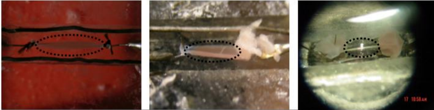
Figure 1. Linear muscle preparations (within dotted ovals) attached to micro-force transducers for functional measurements. Left: isolated extensor digitorum longus (EDL) muscle; Middle: isolated diaphragm muscle; Right: isolated cardiac trabecula. All muscles are superfused with modified Krebs-Henseleit solution, and continuously oxygenated.
